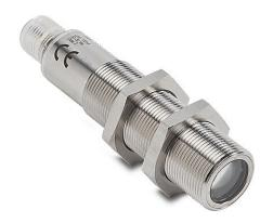
AutomationDirect photoelectric sensor, tubular, threaded, 316L stainless steel housing, through-beam receiver, 20m sensing distance, 10-30 VDC operating voltage, selectable light-on/dark-on, NPN, 4-wire, 4-pin M12 quick-disconnect.
